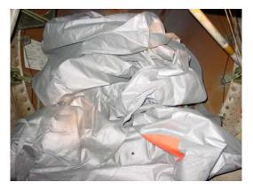
The slide and hardware were removed from the aircraft for examination. There was no evidence of any punctures in the slide; however, there were marks consistent with rubbing of elevator control cables. Additional evidence was found to indicate that a catwalk railing was broken and impinged upon elevator control cables. The slide and hardware will be sent to the manufacturer for detailed examinations supervised by the NTSB.
